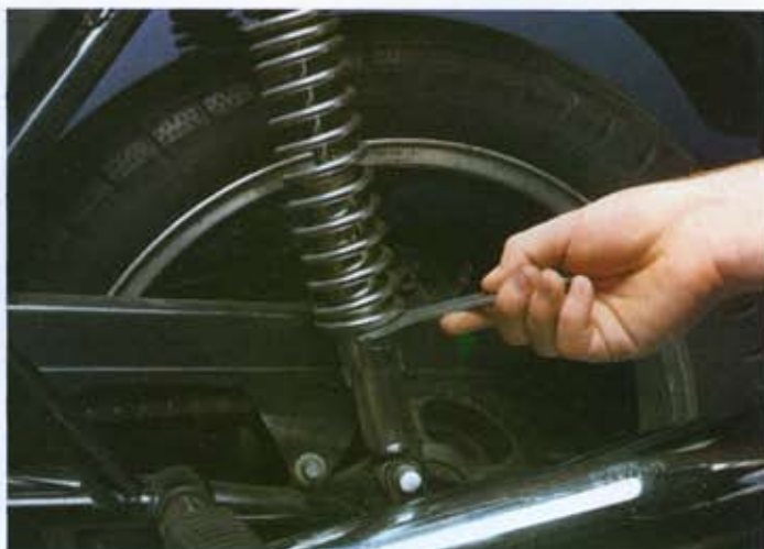
As usual, spring pre-load adjustment is done by C-spanner on the base of the shock absorber
