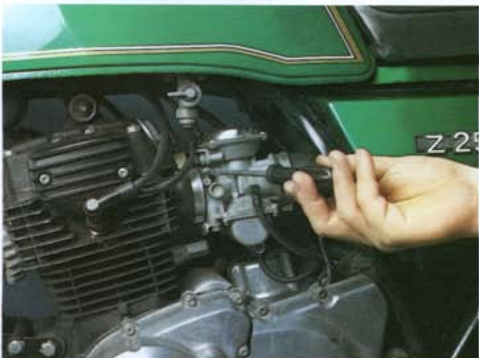
It is unlikely that the carburettor settings will need to be altered. If they do, always adjust with the engine warm
