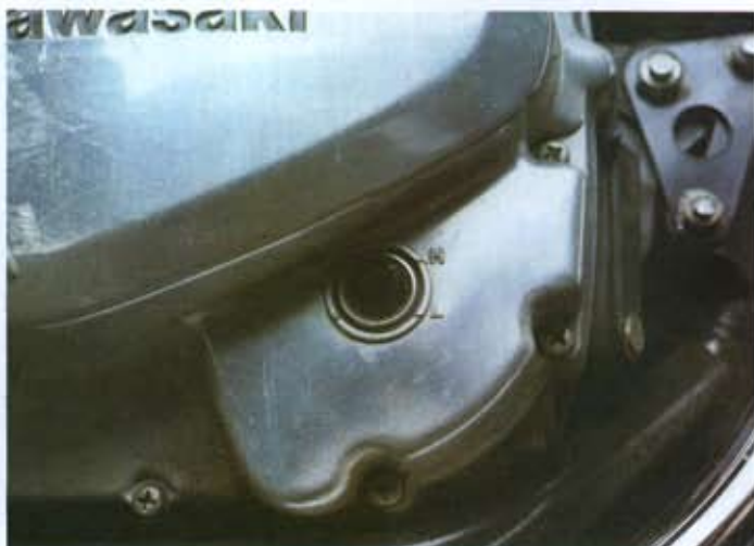
Oil level checking is easy thanks to the window on the right of the engine case. Check with the bike level
