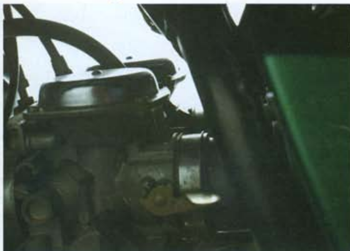
Adjustment of the idle speed is performed simply with the adjuster knob visible between the two carbs
