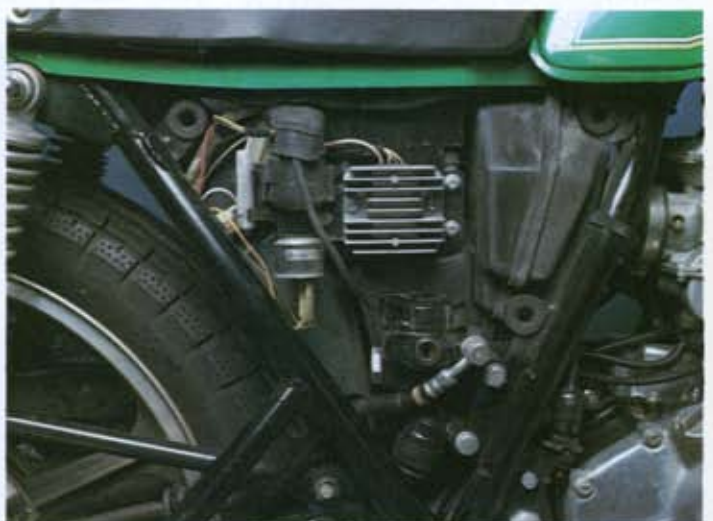
Nestling in among the stiff (though poorly welded) frame members are bike electrics and the rear brake cylinder
