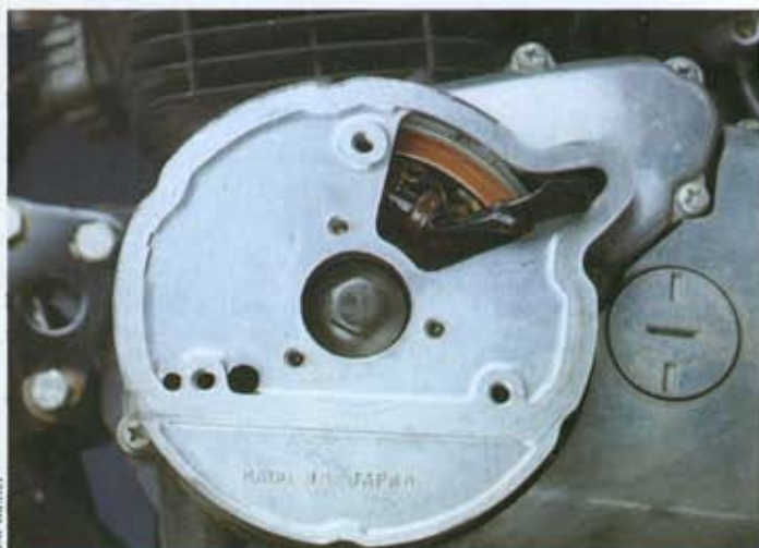
For timing checks, the marks are visible through the window in the cover. Turn the crankshaft by this bolt
