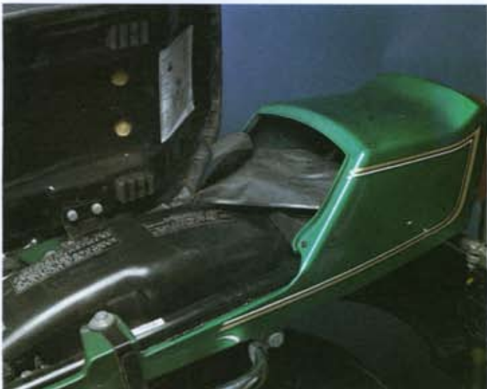
The rear of the seat conceals the very useful little hump under which is a space for the stowing of small items
