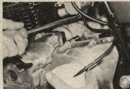
19. Undo the float bowl drain screws in order to flush out any sediment collected in them. Catch the petrol in a small container.
