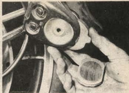
31. Remove the brake pads and inspect for wear. They should be changed if the material has worn down to the red line on the pad.
