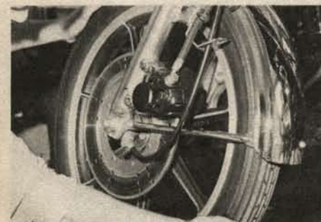
27. Check the wheel bearings for play by pushing and pulling on the rim. They cannot be adjusted, only renewed.
