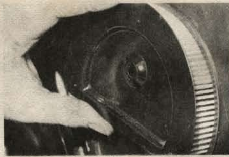
17. Remove the air filter and clean it using a high flash point solvent. Renew after five cleanings. Do not soak in oil.
