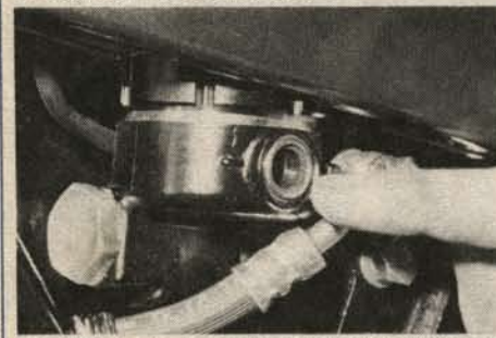
25. Check the level of both hydraulic brake fluid reservoirs. They both have a small sight-glass for this purpose.
