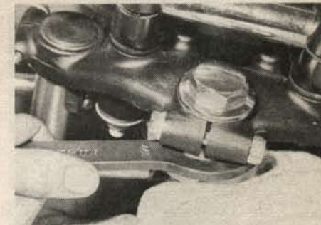
29. If any play is felt it can be taken up by releasing the locknut and using a 'C' spanner on the head race.
