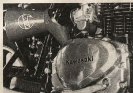
8. Refill with 10W/40 or 20W/50 motor oil until it shows in the sight glass. Run the engine, check the level, and top up if necessary.
