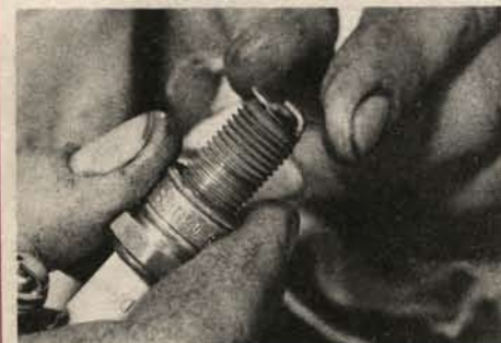
10. Remove both spark plugs and clean and gap them. They should be set to 0.7-0.8mm. Renew them every 6,000 miles.
