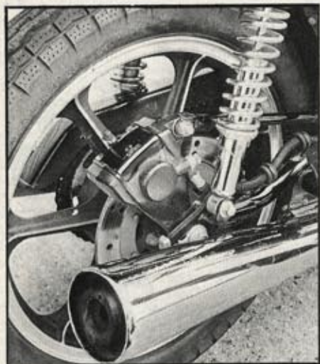
Here's another — the damper. Spring rate and damping are well matched for a good ride. Zorst wails nicely at high revs.
