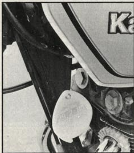
If it's not stiff . . . never mind the tax disc here's part of the reason for good handling. Strategic gusset on a basically stiff frame.
